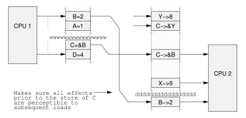
Figure 14.11: Data Dependency Barrier Supplied
