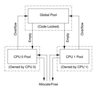
Figure 6.27: Allocator Cache Schematic
