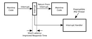
Figure 15.13: Threaded Interrupt Handler
