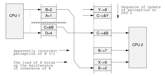
Figure 14.10: Data Dependency Barrier Omitted
