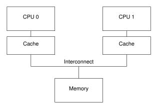
Figure 14.1: Modern Computer System Cache Structure
