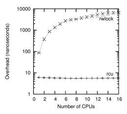
Figure 9.35: Performance Advantage of Preemptible RCU Over Reader-Writer Locking
