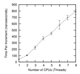
Figure 5.3: Atomic Increment Scalability on Nehalem
