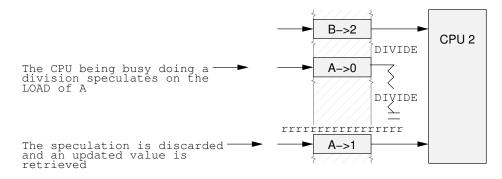
Figure 14.18: Speculative Load Cancelled by Barrier
