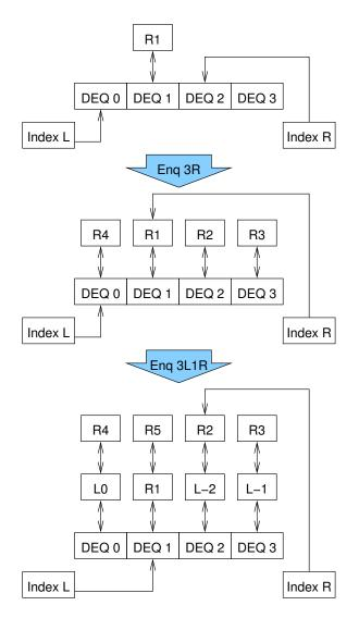
Figure 6.8: Hashed Double-Ended Queue After Insertions
