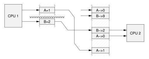
Figure 14.12: Read Barrier Needed
