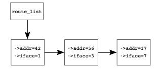
Figure 9.1: Pre-BSD Packet Routing List
