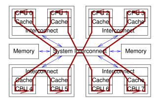
Figure 5.4: Data Flow For Global Atomic Increment
