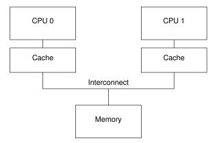
Figure C.1: Modern Computer System Cache Structure
