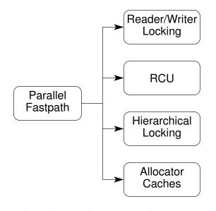
Figure 6.24: Parallel-Fastpath Design Patterns
