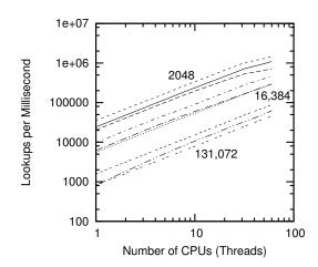
Figure 10.29: Overhead of Resizing Hash Tables
