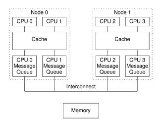
Figure C.8: Example Ordering-Hostile Architecture
