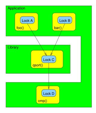
Figure 7.6: Layered Locking Hierarchy for qsort()
