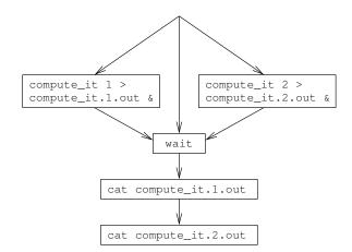
Figure 4.1: Execution Diagram for Parallel Shell Execution
