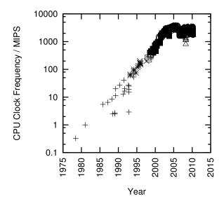
Figure 2.1: MIPS/Clock-Frequency Trend for Intel CPUs
