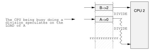
Figure 14.17: Speculative Load and Barrier
