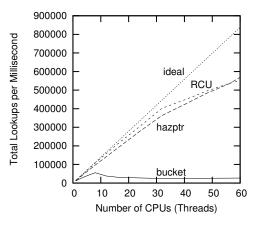
Figure 10.14: Read-Only RCU-Protected Hash-Table Performance For Schrödinger's Zoo, Linear Scale
