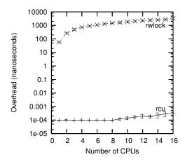
Figure 9.34: Performance Advantage of RCU Over Reader-Writer Locking
