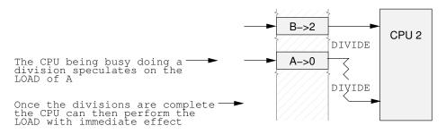
Figure 14.16: Speculative Load
