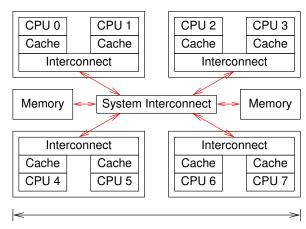
Speed–of–Light Round–Trip Distance in Vacuum for 1.8GHz Clock Period (8cm)
