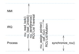
Figure 9.46: RCU API Usage Constraints
