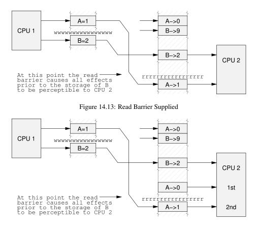
Figure 14.14: Read Barrier Supplied, Double Load
