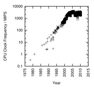
Figure 6.14: MIPS/Clock-Frequency Trend for Intel CPUs
