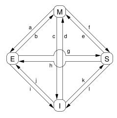
Figure C.3: MESI Cache-Coherency State Diagram
