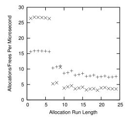
Figure 6.32: Allocator Cache Performance
