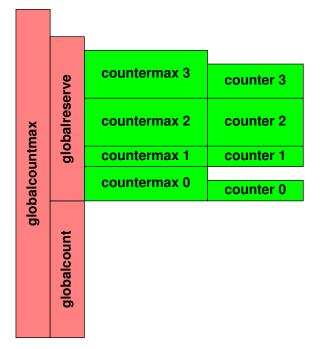
Figure 5.11: Simple Limit Counter Variable Relationships
